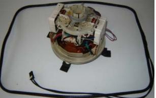
9 & 10 CRT Yoke (centre) & Degaussing coils
