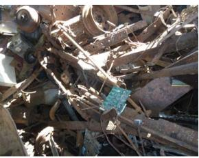
PCB mixed in with scrap steel for baling
