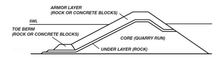
Figure 19: Conventional Multi-Layer Rubble Mound Breakwater Source: (Cummings, et al., 2012)
