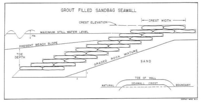
Figure 215 Design of sandbag seawall in Kiribati. (Source: Holden (1992))
