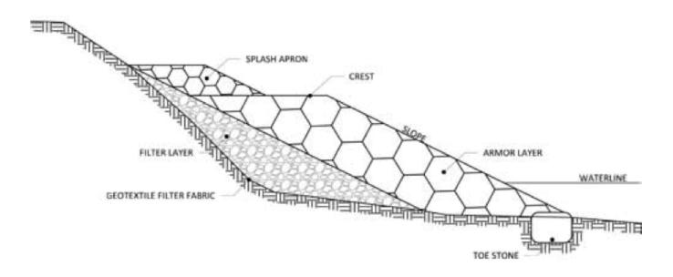
Figure 15: Typical Rock Revetment Section Source: (ODNR, Office of Coastal Management, 2011)
