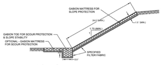
Figure 16: Reno Mattress Section Example Source: http://www.terraaqua.com/bank-paving.php [Accessed 11 February, 2015]
