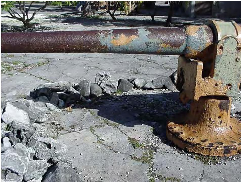
Photo 11 12cm Gun showing the zinc-rich primer area painted on the barrel in 1992.
