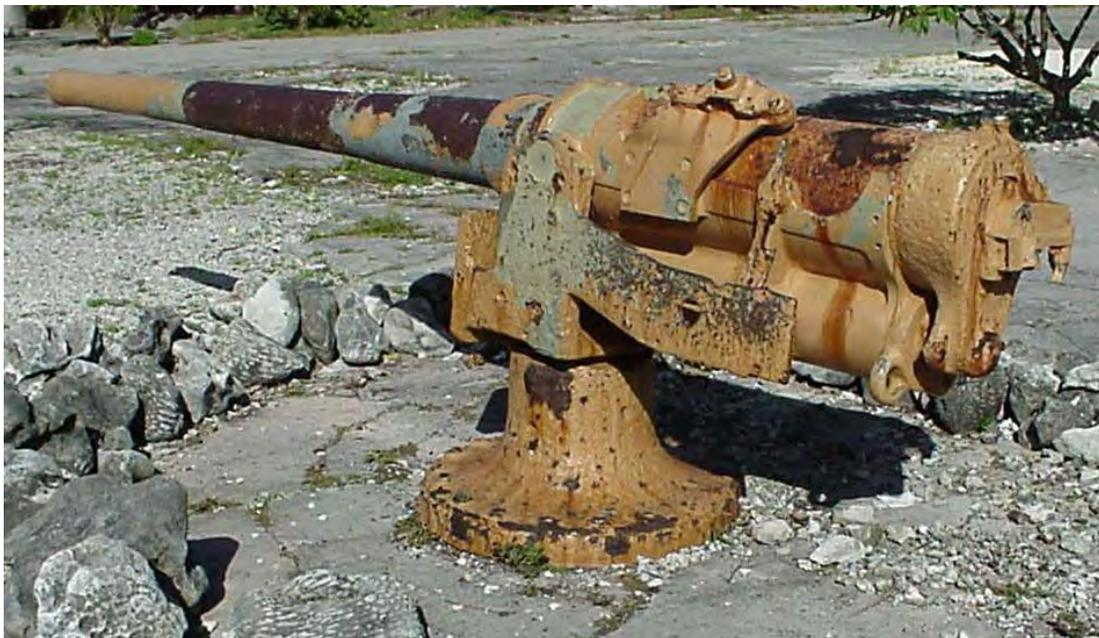
Photo 9 12cm Gun showing the zinc-rich and red-lead primer areas painted in 1992. The light green color at the opposite ends of the gun is the red-lead primer. The blue color in the middle is the zinc-rich primer.
